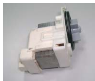
Pompe de vidange 30W – 17-21L/sec – 143ohm \pm 7\% - Protection thermique 120C°
